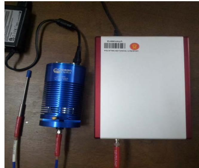
Fig. 2: (a) The illustration of the NIR measurement setup, (b) the actual NIR Spectroscopy setup
